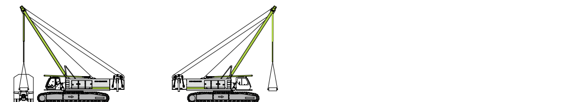
Unloading and assembly of central counterweight
